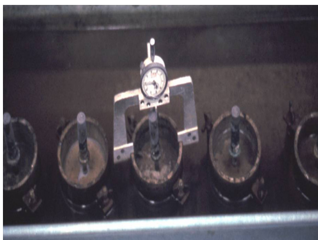
Fig. 3. Parallel volume expansion test.
